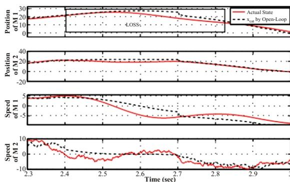
Fig. 4. Highlighted view of data loss region
