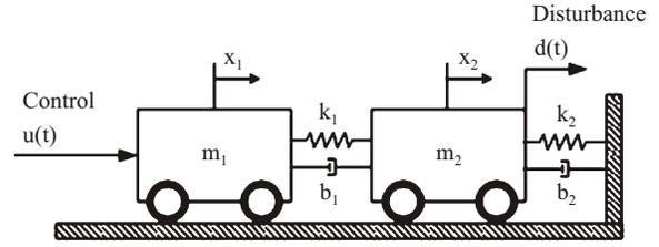
Fig. 2. Mass-Spring-Damper system
