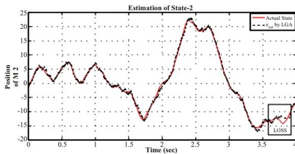
Fig. 9. Performance of LGA for data loss 3.7 3.9 sec
