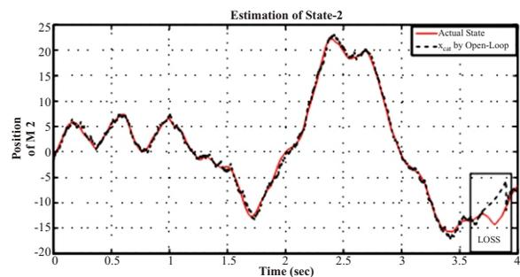
Fig. 7: Open Loop Estimation for data loss from 3.7 to 3.9 sec
