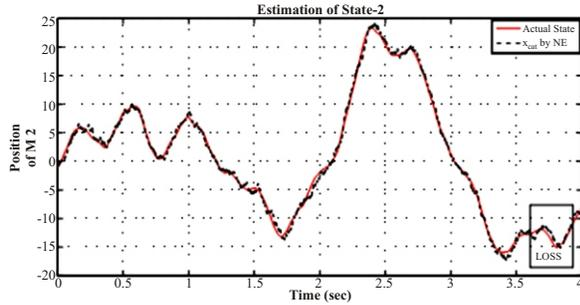
Fig. 8. Estimation through NE for data loss 3.7 - 3.9 sec
